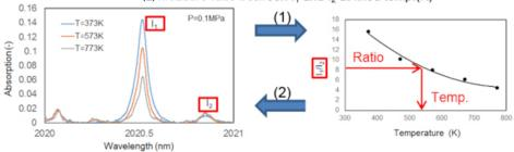
(2) Calculate temperature from the ratio curve (I1/I2).
